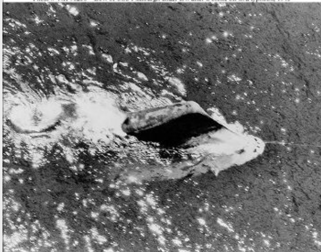
Photo # NH 98249 USS Pittsburgh at Guam after losing her bow in a typhoon
