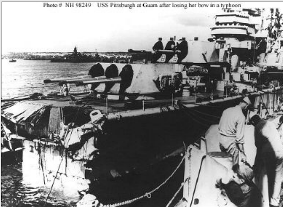
Photo # NH 98249 USS Pittsburgh at Guam after losing her bow in a typhoon
