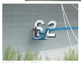
**USS Iowa class battleships:** \* This photo provides reference to the size of the hull numbers as you point them out to tours. The number "62" shown here is **8 feet high.** Iowa Class battleships originally included six ships to be numbered & built as follows:
