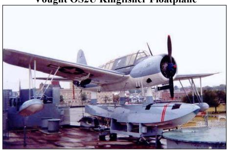
After a sortie, the planes would land on the water close to the ship and taxi onto a recovery sled being towed by the ship. The plane would then be hoisted aboard by the stern crane.
